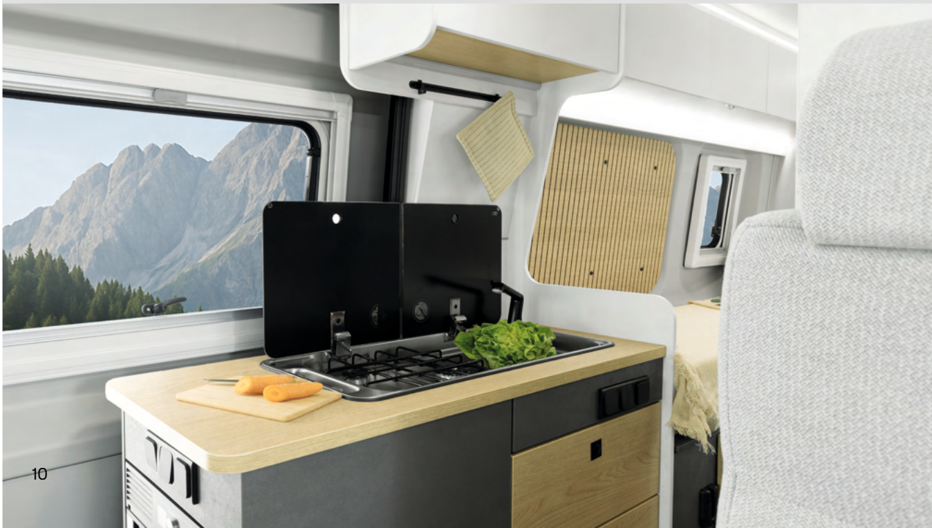
Integrated sink and 2-burner stove with piezo ignition and covers
